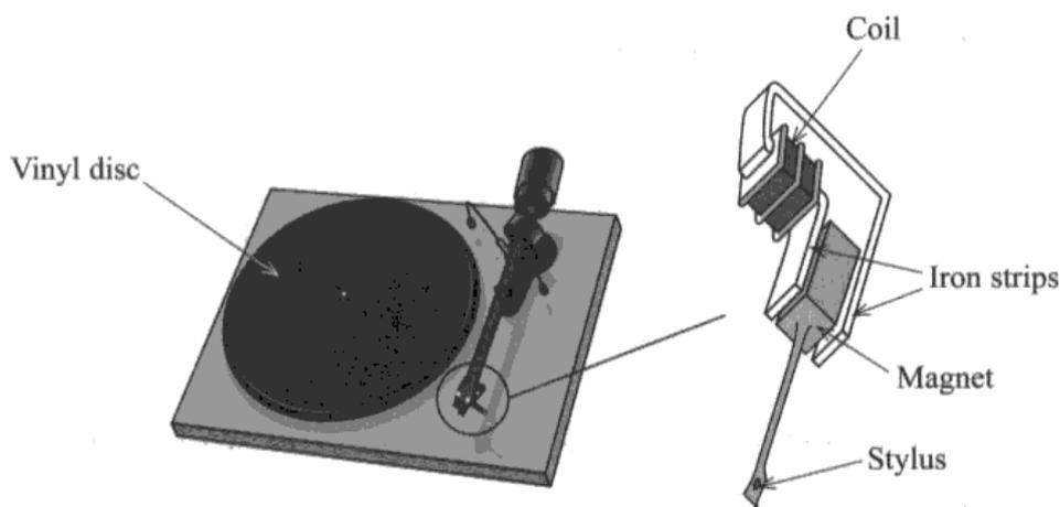
The stylus is attached to a small magnet which is near to a coil of wire. When the stylus vibrates, there is a potential difference across the terminals of the coil.
