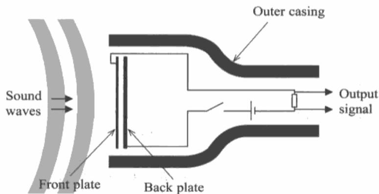
The sound waves cause the flexible front plate to vibrate and change the capacitance. Moving the plates closer together increases the capacitance. Moving the plates further apart decreases the capacitance.
