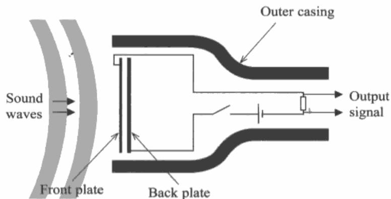
The sound waves cause the flexible front plate to vibrate and change the capacitance. Moving the plates closer together increases the capacitance. Moving the plates further apart decreases the capacitance.
